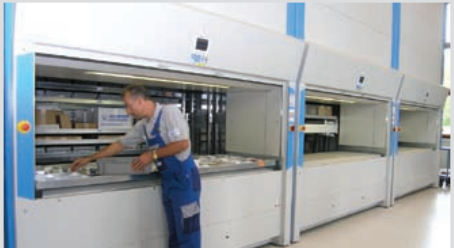
Warehouse lift with height measurement using optical sensors and securing of the removal area
